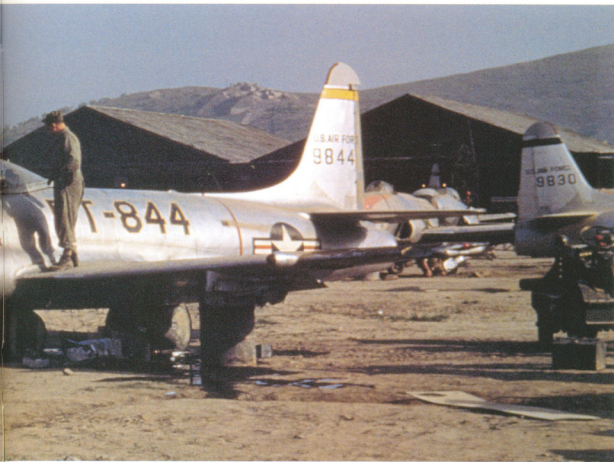
LEFT BELOW Maintainers had their hands full repairing battle-damaged F-80s in time for the unit's next mission. This 8th FBS machine seems to have suffered a nose gear failure on landing at Taegu, which has necessitated the removal of the whole forward section of the jet. The repair work is already well underway, and chances are that the F-80 was ready to fly another mission within 48 hours of the accident taking place. The other F-80 shown in this view is a blue-trimmed 7th FBS jet, this unit being co-located at Taegu in the late spring of 1951 (Nat King)
